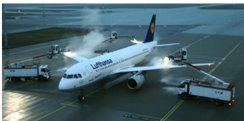
Figure 5. Freezing point depression is exploited to remove ice from the control surfaces of aircraft [5].
