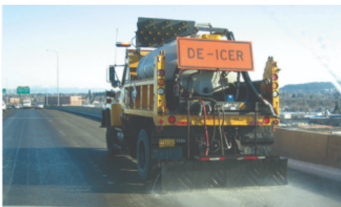
Figure 4. Freezing point depression is exploited to remove ice from roadways [5].
